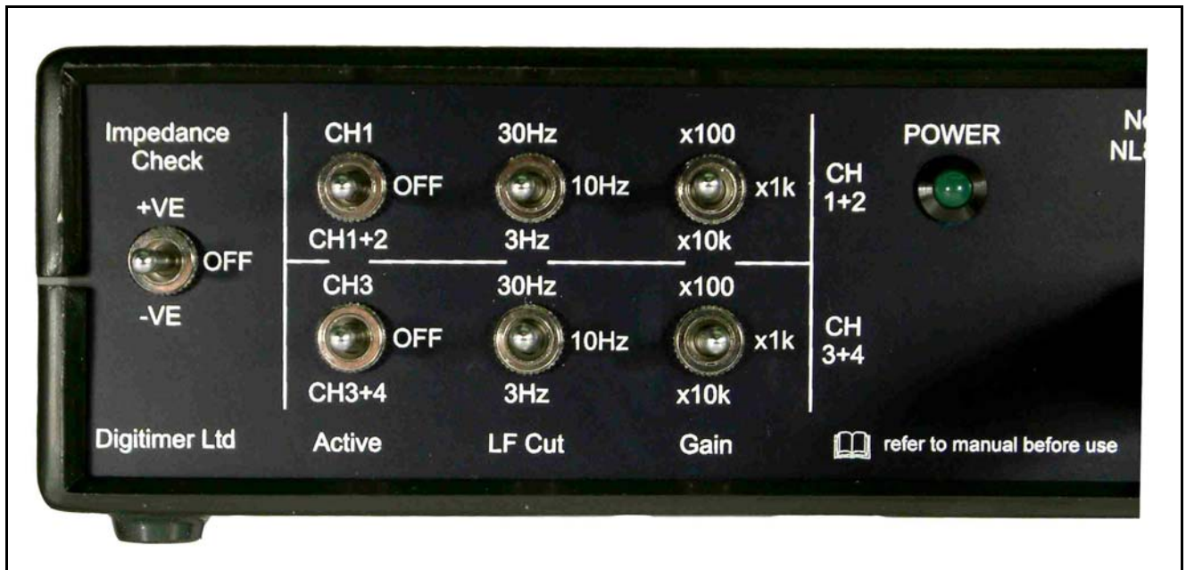
The left hand side of the Rear Panel of the NL844 showing the controls for Impedance Check, Channel Enable, LF-cut and Gain. Also the power LED. The cable connection to the NL820A is off to the right-hand side.
