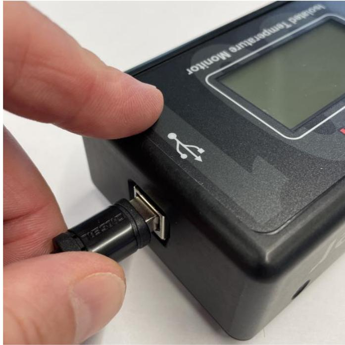
3. Confirm successful connection by checking the LCD screen is illuminated and displaying a temperature value, which changes when the thermistor is warmed.
