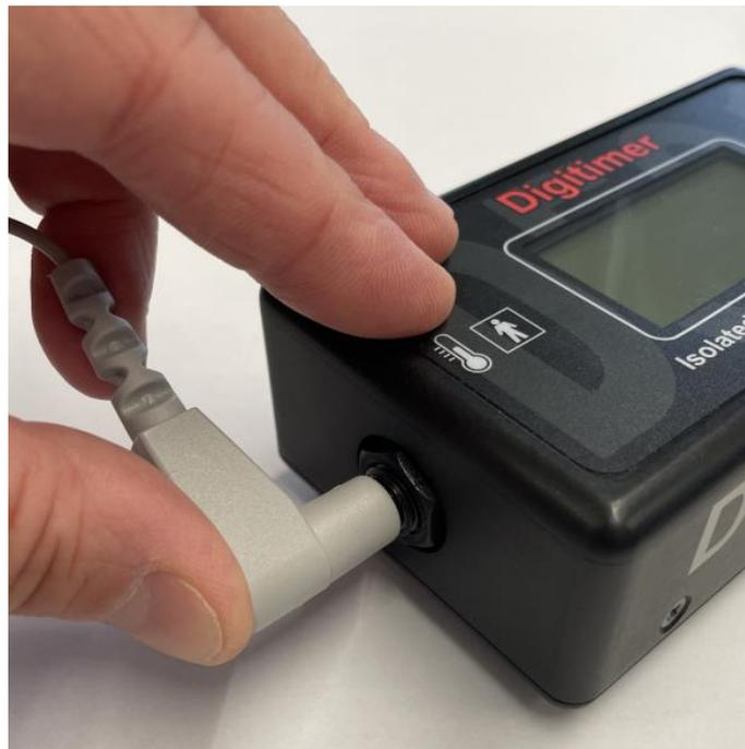
2. Connect the USB-B end of the supplied USB cable to the USB-B socket on the right of the D501 and the other end to a standard USB-A port on your Windows PC. Ensure the plug is fully inserted as shown below.
