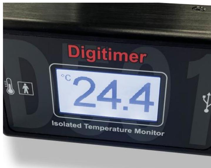
4. If the LCD screen fails to illuminate and remains blank, this may indicate that the D501 is not receiving adequate power. Check the PC is powered ON and try a different USB port or an externally powered USB hub.
