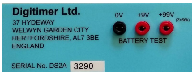
Figure 6 - Battery test sockets are provided to test the output and control batteries without disassembling the DS2A.
