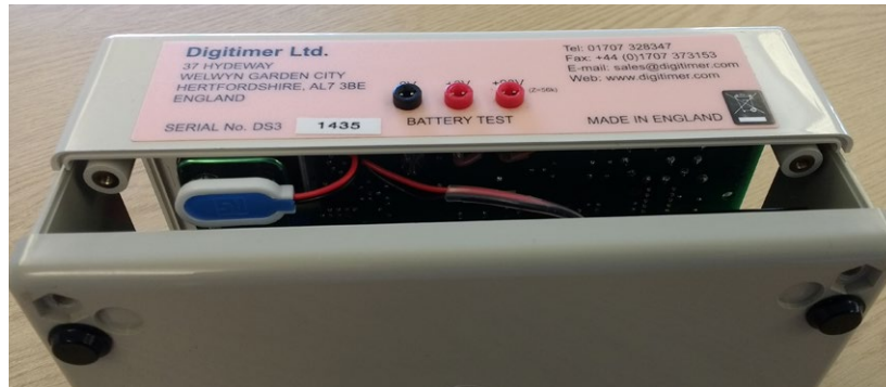
Figure 7 - With screws removed, the case halves can be slid apart.
