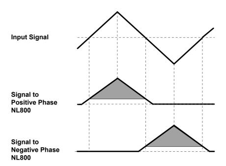
This diagram shows a bipolar input signal and the signals to the two NL800's. The solid areas indicate where each NL800 operates. Note that the DC offset of each NL800 is automatically added to the input signal before being applied to the NL800.
