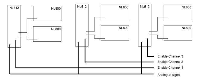
With this arrangement, you can control multiple bipolar channels one at a time from a PC card with a single analogue output and multiple digital control lines being used to enable the required channel.
