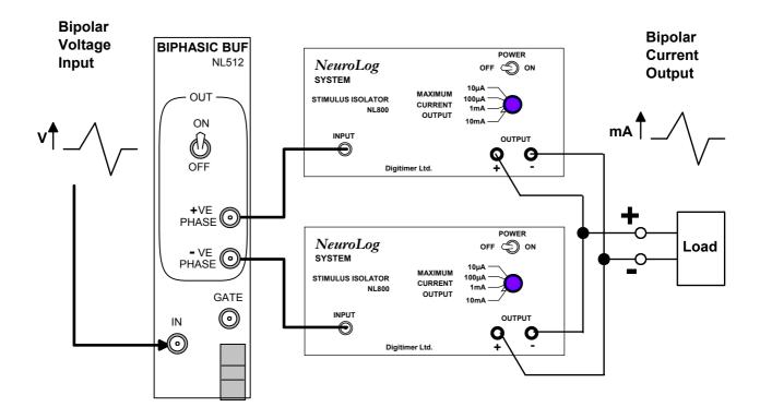
With this connection, a bipolar voltage input signal will produce an isolated bipolar current output through the load (preparation).
